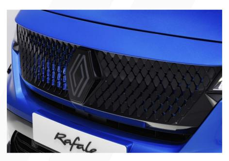
The All-new Renault Rafale's novel radiator grille is built around the brand's hallmark diamond. It is made up of a constellation of small diamonds that arrange space in three dimensions around the emblem in the middle.
