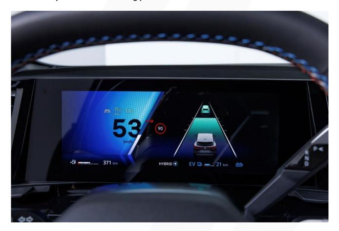
For optimal, stress-free driving pleasure, the All-new Renault Rafale comes with 32 advanced driver assistance systems (ADASs) divided into three categories: driving, safety and parking. And it now includes Intelligent Speed Assist (ISA), a system that automatically alerts the driver if the car's speed exceeds the limit it reads on road signs.
